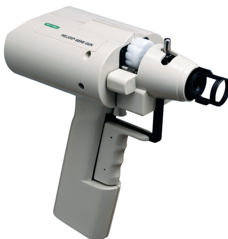
Fig. 6.3 A Helios gene gun. It uses a low-pressure pulse of helium to sweep DNA, RNA, or protein-coated gold particles from the inner wall of a small plastic cartridge directly into target cells. (From Bio-Rad Inc. With permission.)
